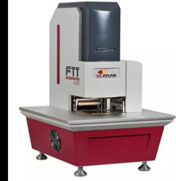
14. Testing device for determination of fabric comfort / touch
