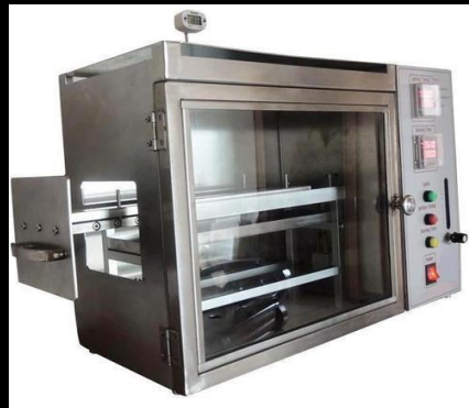
7. Horizontal Flammability Test Chamber
